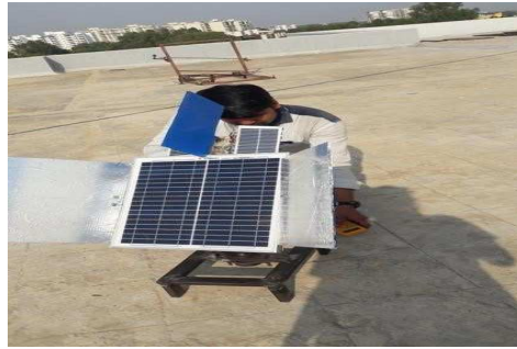
Figure 3: Sun Tracking with Reflectors
