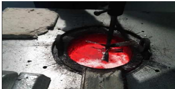
Figure 2: Stirring of AA2024 with B4C Reinforcement
