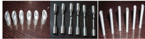
Figure 2. Specimens used for Hardness, Tensile and Wear test.
